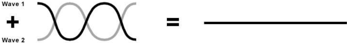
When the Crest of Wave 1 meets with the trough of Wave 2 there is deconstructive interference and no light appears because they effectively cancel each other out.
