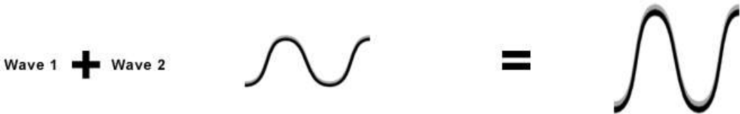
When the Crests of Wave 1 and Wave 2 meet together then there is constructive interference and the light is intensified.
